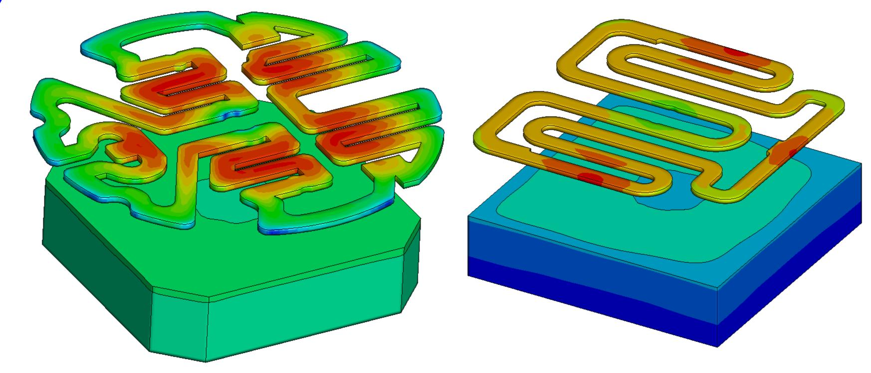
> The high temperature of the round top heater is concentrated in the center, and the temperature gradually decreases along the radial direction.
