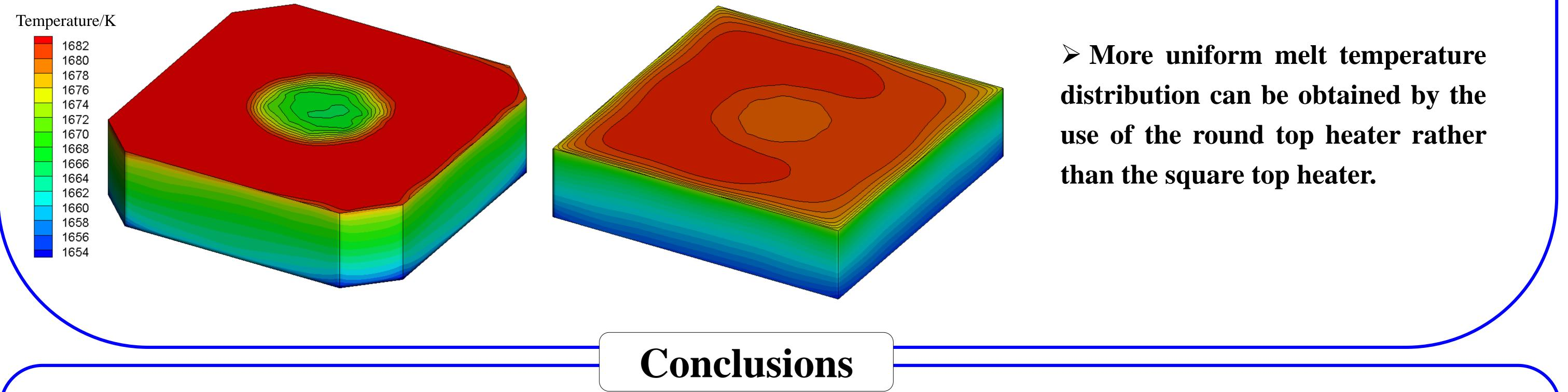
1. The use of octagonal crucible with the round top heater is beneficial for obtaining high efficiency monocrystalline silicon ingots.
